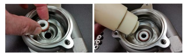
Place the ceramic portion of the seal, boot down into the housing. Use small amount of dish soap.
