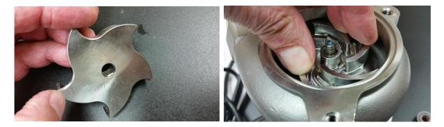
Note the impeller has a "D" cut hole which aligns with the motor shaft flat.
