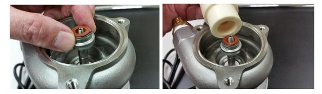
Also lube the protective shield covering the threads, slide the seal on the shaft, use open side of the tool.
