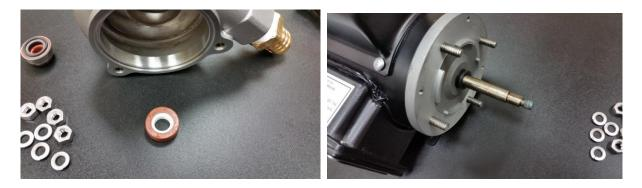
With two seal parts removed and housing off of the motor, the new motor can be put into the assembly.
