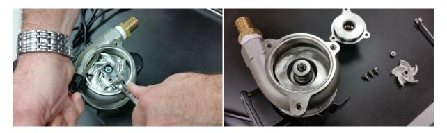
Brace the impeller against a screwdriver to remove the locknut holding the impeller to the shaft.
