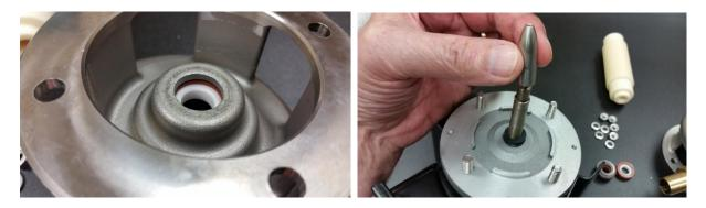
Turn the housing over, check that seal and boot are fully seated in housing, place protective shield over the threads on the motor shaft.
