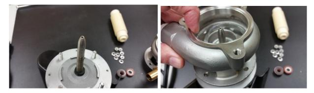
Carefully place the housing on the motor, align the housing correctly and slide it over the 4 attachment studs.
