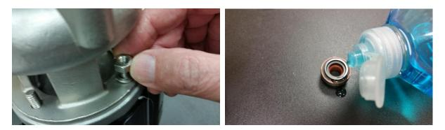
Place lock washers and nuts on the studs and tighten. Place small amount of soap on black portion of seal.
