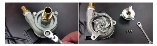
After removing the pump from the machine, remove 3 bolts and lock washers holding pump cover on.
