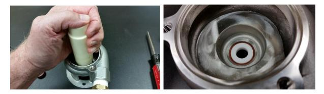
With tool 088-1092 press the ceramic firmly to the bottom of the housing.
