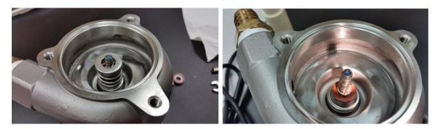
Look closely at the shaft to see the side machined with a flat; this must be aligned with impeller.
