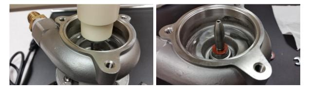
Carefully press the seal down the shaft until seated against the white ceramic portion of the seal. Do not pound or hammer on the installing tool, this could break the ceramic portion.
