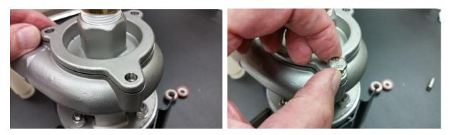
Align the cover, insert the ¼-20 SS bolts and lock washers, tighten firmly. Remove the plug on the end of the motor cord and attach motor wires to the original wires of the machine control for the drain pump.
