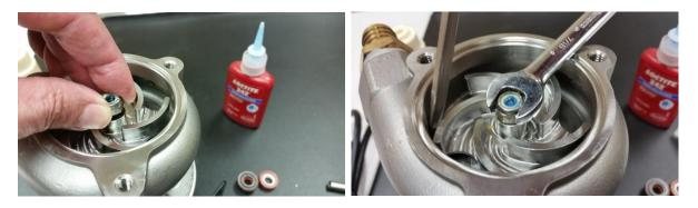
Place one drop of Loctite on shaft threads. Brace impeller with a screwdriver and fasten locknut 098-2507 to hold impeller securely to the motor.
