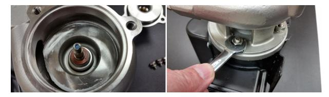
Take the spring and cap out, remove the 4 nuts and washers holding the housing to the motor.
