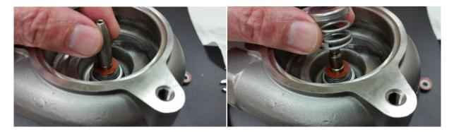
Remove the protective shield, place the spring over the seal collar with the cap on top.
