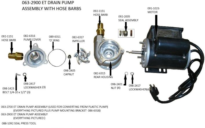
098-9009 HOSE CLAMP (NOT SHOWN) 7 PER MACHINE 093-1051 HOSE, (BULK) 78 1/2" PER MACHINE
