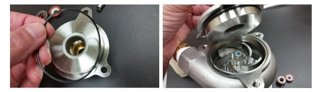
Place O-ring gasket 089-6311 on the pump cover and place into the pump housing
