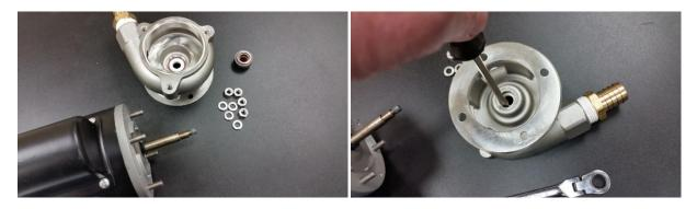
Lift the pump housing off the motor; from the back of the housing push the ceramic portion of the seal out.
